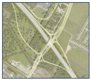
The Pecue Lane DDI provides a higher level of operational efficiency and is a safer alternative to a conventional diamond interchange. It will consist of three thru lanes in each direction with raised medians and sub-surface drainage.
